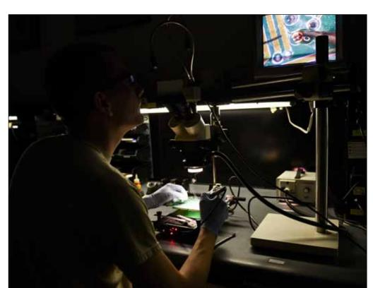
Left: U.S. Air Force Staff Sgt. James Lott, an Air Force Repair Enhancement Program circuit card technician assigned to the 509th Maintenance Group, uses the soldering station to replace a through-hole mounted resistor to fix a circuit card at Whiteman Air Force Base, Mo., Nov. 17, 2016. The display screen enhances Lott's view of the item to check for damages, look for Foreign Object Debris (FOD), and check for cleanliness.
