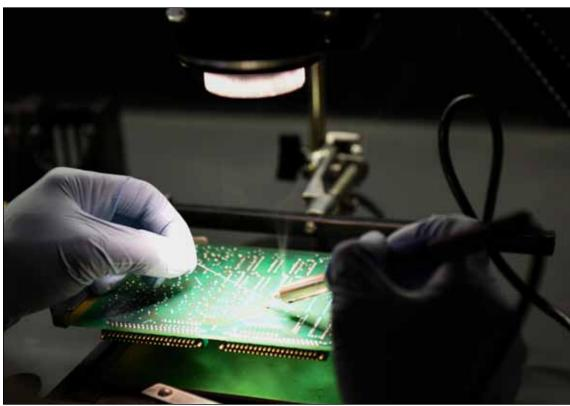
U.S. Air Force Staff Sgt. James Lott, an Air Force Repair Enhancement Program circuit card technician assigned to the 509th Maintenance Group, works at a soldering station to fix a circuit card at Whiteman Air Force Base, Mo., Nov. 17, 2016. A heater is located under the circuit card to help solder joints and reduce the chance of thermal shock on components.
